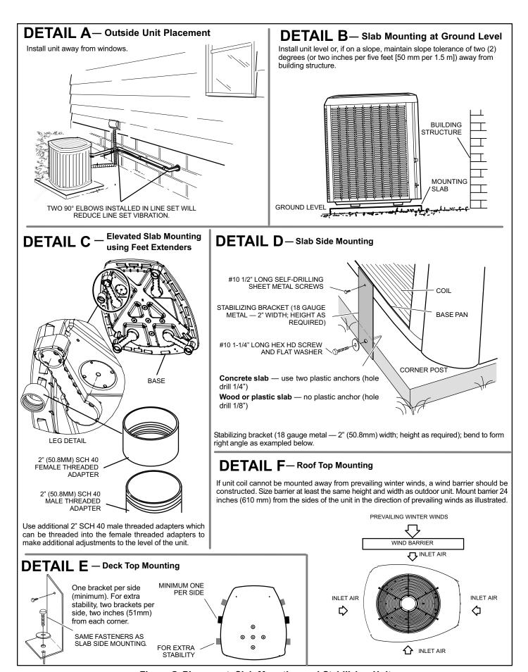
Figure 5. Placement, Slab Mounting and Stabilizing Unit
